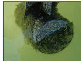
Before cleaning the face of the transducer.
