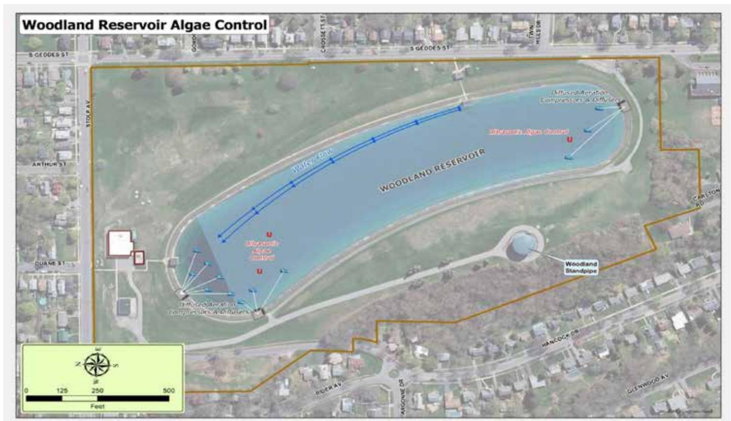
Figure 5. Woodland Reservoir algal control device arrangement.
